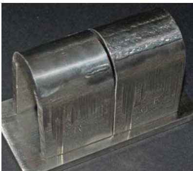
Guided Bend Test (Root & Face Welding Coupons)
