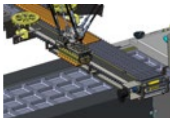
Robot uses vacuum to pick product pieces at once and moves toward the pocket.
