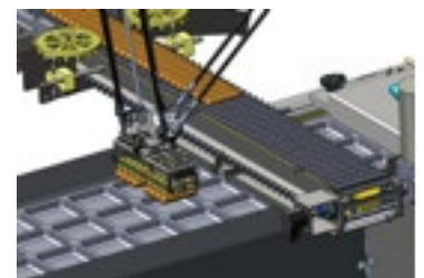
As the robot moves toward the pocket, the end effector groups and separates the product pieces prior to placing them in the pocket.
